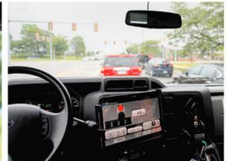
A van in a program to test the safety benefits of cars communicating with one another and their surroundings is equipped with a camera, top right, a rearview mirror that signals when a driver stops ahead and a digital display linked to traffic lights. Joshua Lott for The New York Times
