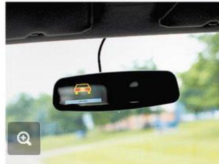
A van in a program to test the safety benefits of cars communicating with one another and their surroundings is equipped with a camera, top right, a rearview mirror that signals when a driver stops ahead and a digital display linked to traffic lights. Joshua Lott for The New York Times
